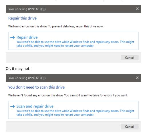
6. Scan the drive regardless. Errors may be repaired even if they were not detected initially.
